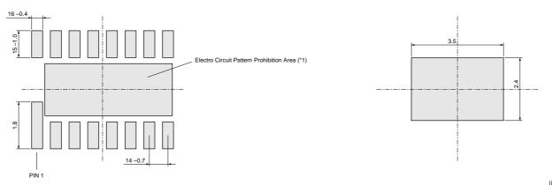
(\*1) Do not make the electro circuit pattern at the prohibition area to prevent contact with the central terminals of product's back side and to prevent interference with the other signal. (Prohibition area: the central hatching area at 1st layer)
