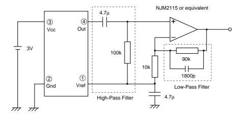
The hiph-pass filter's cut-off frequency in this circuit is approx. 0.3Hz. The low-pass filter's cut-off frequency in this circuit is approx. 1kHz.
